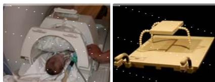
Figure 1. CMR coils used for imaging newborns. Quadrature head coil (left panel), custom built newborn multichannel – array coil (right)
