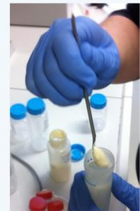
Illustration from left to right: Kryo centrifugation for 15 minutes at 2° C; milk tubes after kryo centrifugation show the separated milk: fatty cream and skimmed milk; removal of the cream by spoon
