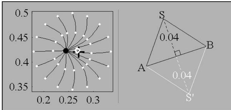
**Figure 4:** Left: A possible alternative interpretation of the data in experiment 2 (here for the pink background, cf. figure 3, top panel) in terms of curved lines of constant hue. Right: Illustration of the choice of infield chromaticities in experiment 3 (see text for details). The black and white lines correspond to two different conditions used for each surround.
