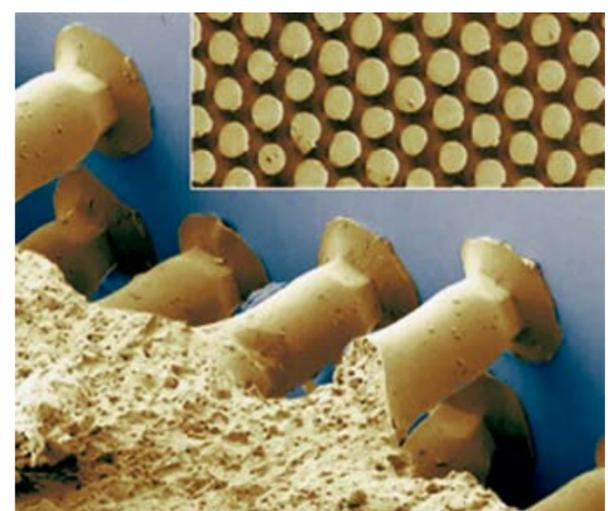
Microscopic image of the biomimetic surface structure of a synthetic adhesive material. The material inspired by the soles of insects feet (in ocher) clings to glass (in blue).
